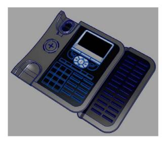
The extension module features 28 keys. One can plug up to 2 extension modules in a row, leading to a total of 10 + 2x28 = 66 possible "multiline" keys.
